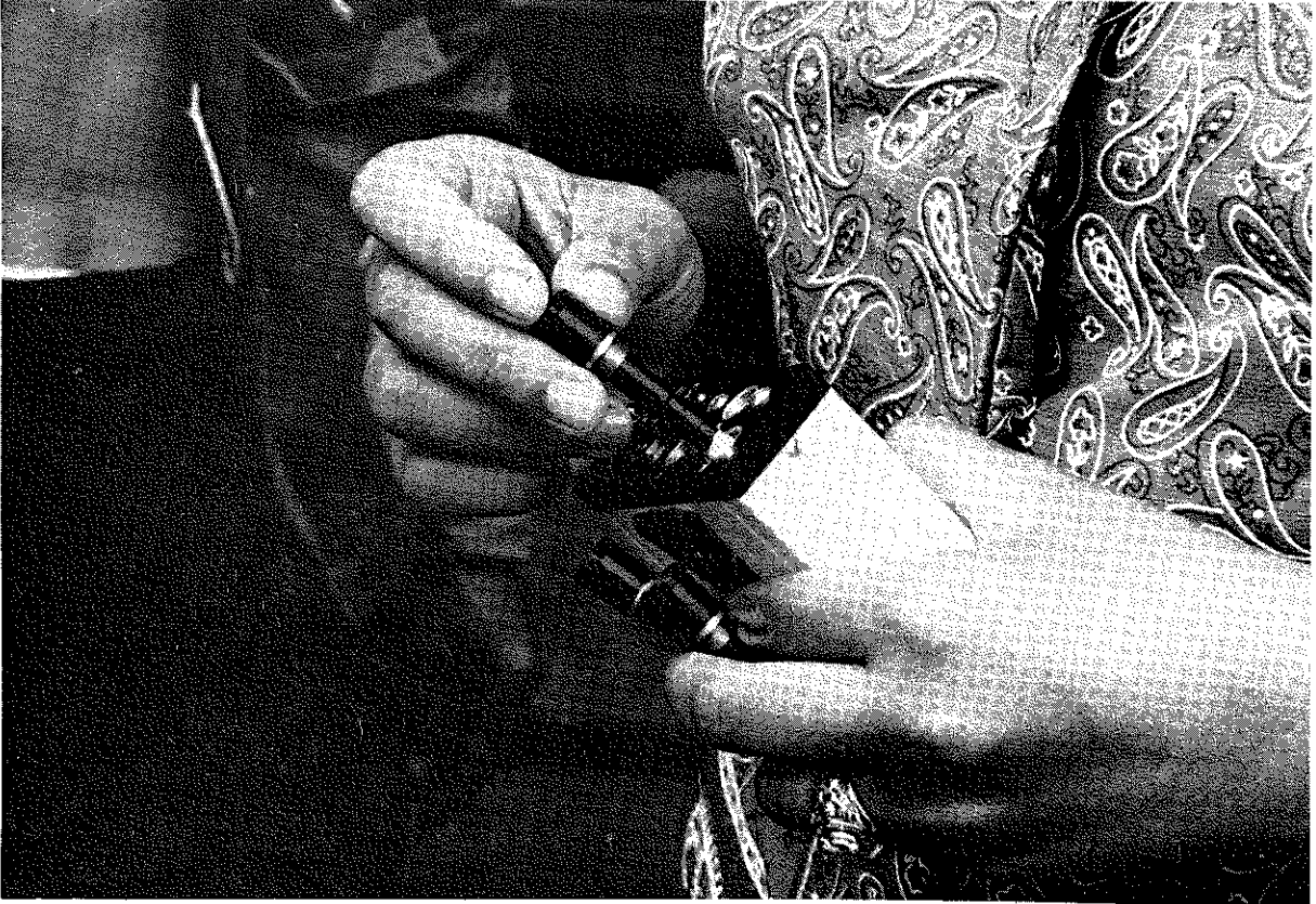
PHOTO 5. INSERTION OF E-CELLS PRIOR TO MONITORING
